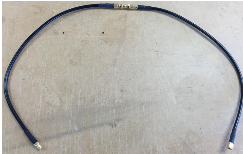
Fig.14 LMR-195 Cable connected using an adapter
