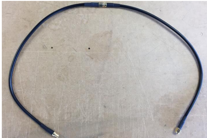
Fig.6 Connected LMR-195 cable
