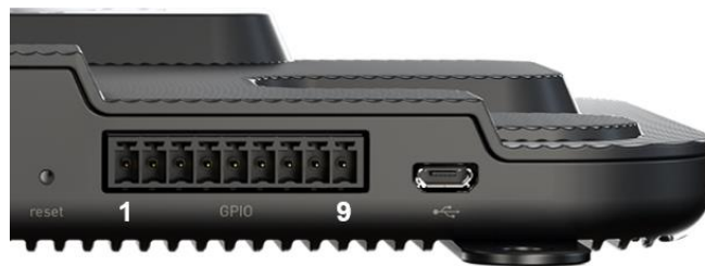
Figure 8: Impinj R700 GPIO Pin Locations
