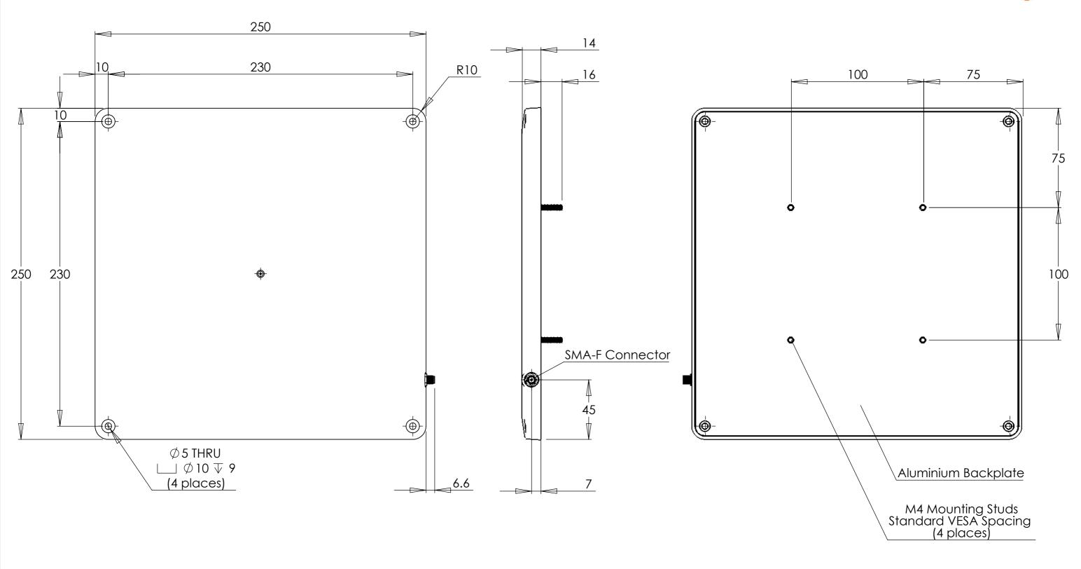
THE INFORMATION CONTAINED IN THIS DRAWING IS THE SOLE PROPERTY OF TIMES-7 LTD. ANY REPRODUCTION IN PART OR AS A WHOLE WITHOUT THE WRITTEN PERMISSION OF TIMES-7 IS PROHIBITED **DESCRIPTION** UNLESS OTHERWISE SPECIFIED TOLERANCES: NO DECIMAL PLACES ± 1 ONE PLACE DECIMAL ± 0.5 A5010 Circularly Polarised Stud Antenna PROHIBITED. DATE: 7-3-25 DRAWN BY: M. Price DATE: 13-3-25 APPROVED BY: P. Wilcock
